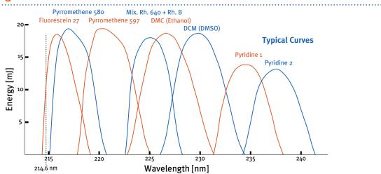
Tuning curves with different dyes, when using approximately 600 mJ @ 532 nm for pumping and 300 mJ @ 355 nm for mixing.
